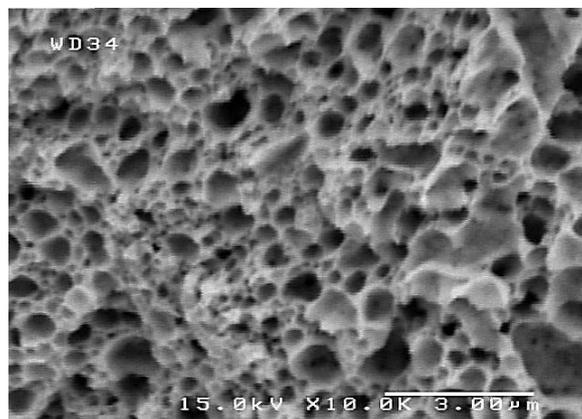
Fig. 5 Typical fracture surface morphology of Cu-0.5 wt.% CNT hot pressed sample.
