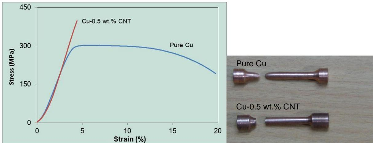
Fig. 4 a) Typical stress-strain curves obtained from the hot pressed samples, and b) fractured samples.
