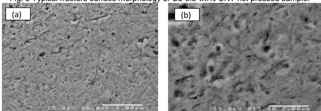
Fig. 6 Cross sectional SEM micrograph of Cu-0.5 wt. % CNT, a) submicron pores and cracks distribution, and b) higher magnification.
