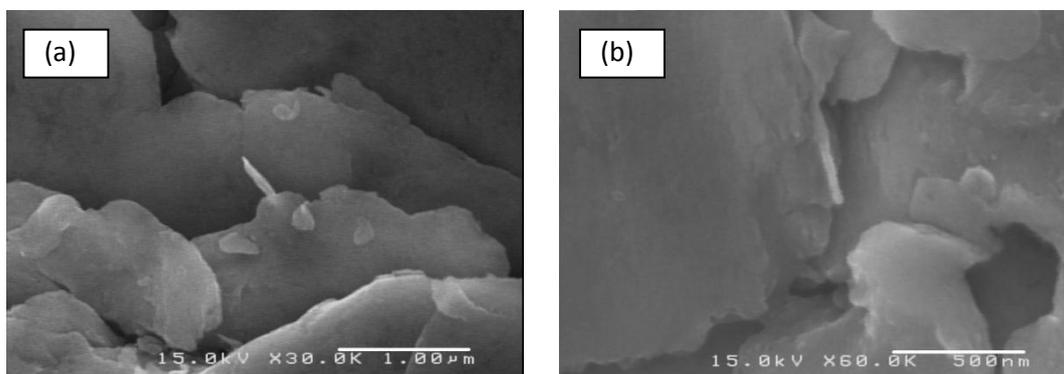
Fig. 3 High magnification FESEM image of powder morphologies after 3 h milling, a) Cu-0.5 wt. % CNT, and b) Cu- 1 wt. % CNT.
