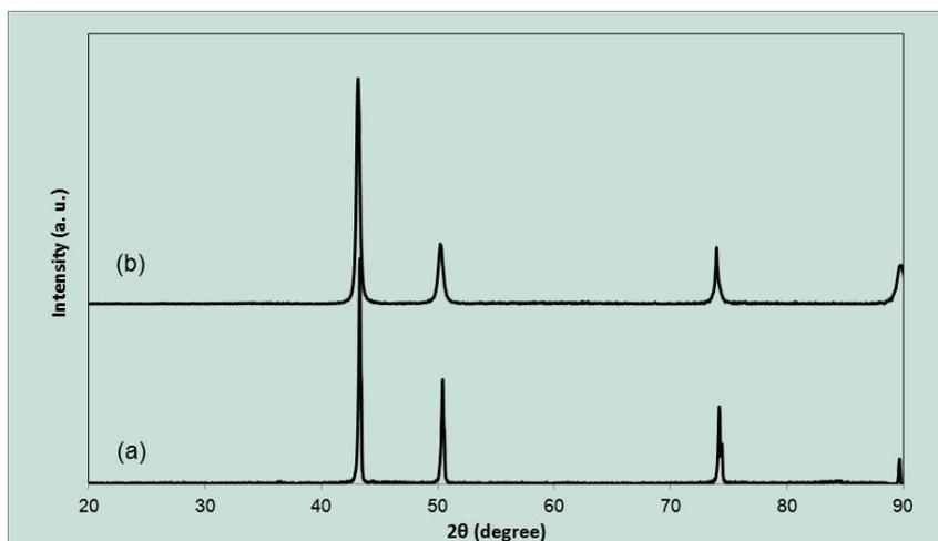
Fig. 8 X-ray diffraction patterns obtained from hot pressed materials a) Pure Cu, and b) Cu-0.5 wt. % CNT.
