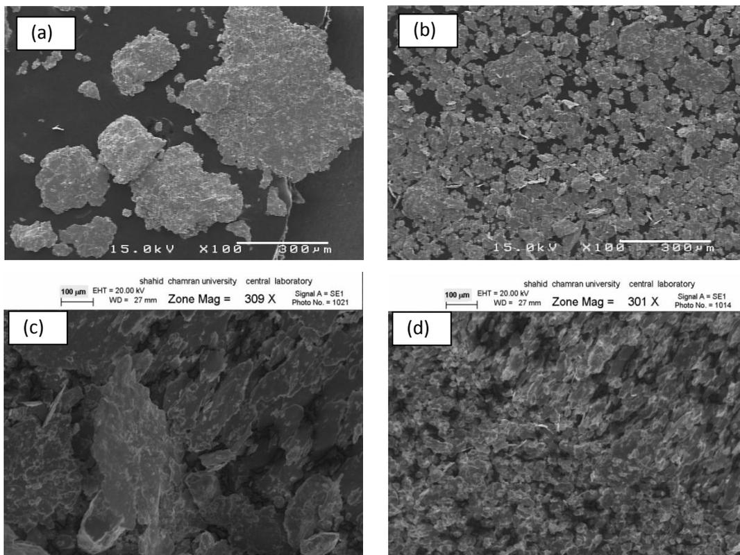
Fig. 2 Morphologies of milled powders, a) Cu-0.5 wt.% CNT after 3h milling, b) Cu-0.5 wt.% CNT after 15h milling, c) Cu-1 wt.% CNT after 3h milling, and d) Cu-1 wt.% CNT after 15h milling.
