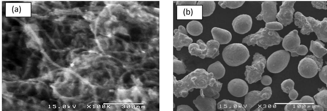
Fig. 1 Morphologies of starting materials, a) MWCNT, and b) pure Cu powder.
