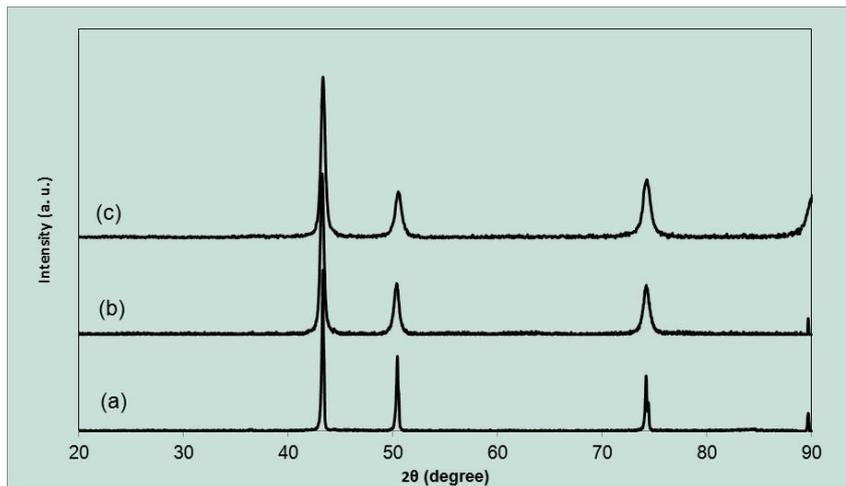
Fig. 7 X-ray diffraction patterns obtained from a) initial Cu powder, b) Cu-0.5 wt. % CNT milled for 3 h, and c) Cu-0.5 wt. % CNT milled for 15 h.
